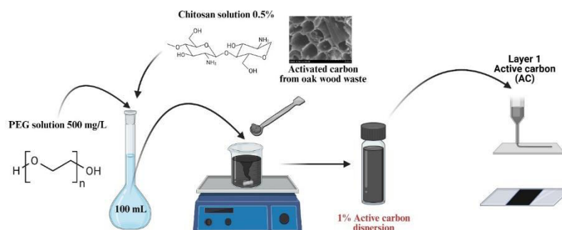
Figure 1. Schematic of the synthesis method for the activated carbon (AC) base layer.
