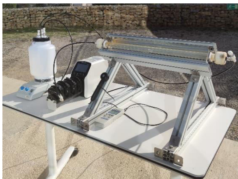
Figure 1. Compound parabolic collector used for solar photo-Fenton experiments.
