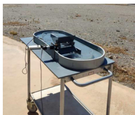
Figure 1. (a) Image of RPR used in this study at CIEMAT-PSA facilities, (b) E. coli inactivation with different FChl concentrations in the dark and under solar radiation.
